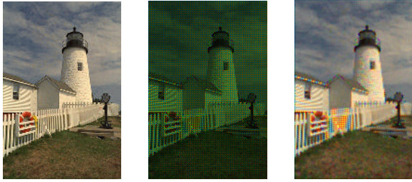
Figure 2: Example of a bilinear interpolation computed with convolution filters. Left: the original image (sub-sampled by a factor of 2 in the horizontal and the vertical direction). Center: one-color per pixel image according to the Bayer CFA. Right: image reconstructed with bilinear interpolation.
