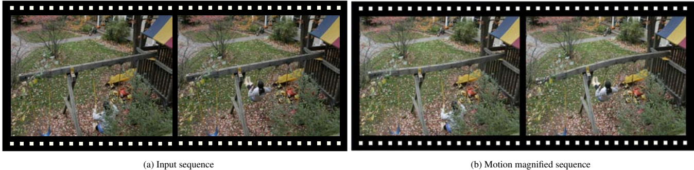
Figure 1: Frames from input and motion magnified output sequence. The algorithm groups the input (a) into motion layers and amplifies the motions of a layer selected by the user. Deformations of the swing support elements are revealed in the motion magnified output sequence (b), magnifying the original motions by a factor of 40.
