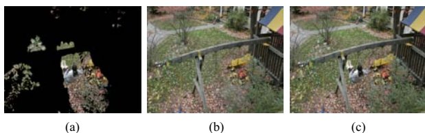
Figure 6: (a) Outlier locations, not well described by our model. Pixel intensities from these locations are passed through from the registered video into the rendered model (b) to yield the final composite output sequence, (c). The user specifies at which depth layer the outliers belong, in this case, above the background and below the other layers.
