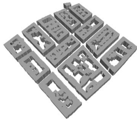
Figure 3. VRML visualization of prismatic models created from the boundary polygons of the building regions from Figure 2.
