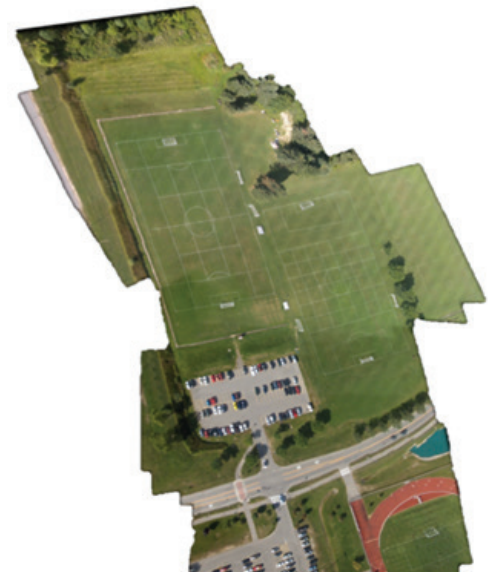
Mosaic resulting from challenging flight over field with straight lines to test the accuracy.
