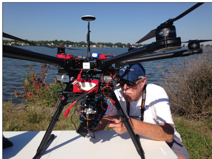
Figure 4: "Papa" Jeff Ring is seen here preparing for a flight to carry the RIT-owned TetraCAM micro-MCA 6 SNAP sensor on Pegasus Environmental's DJI S900 multi-coptor during a recent collaborative experimental flight over soybean fields at Maier Farms.
