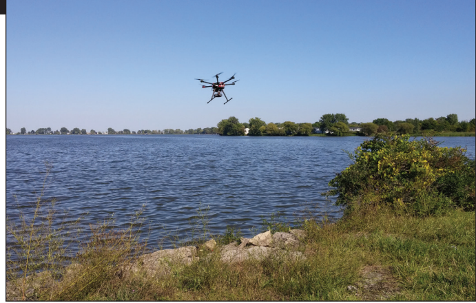
Figure 1: The initial ascent of Pegasus Environmental's DJI S900 and RIT's TetraCAM micro-MCA 6 SNAP sensor during a water quality mapping experiment carried out coincident with a Landsat Thematic Mapper over flight at the southern end of Long Pond.
