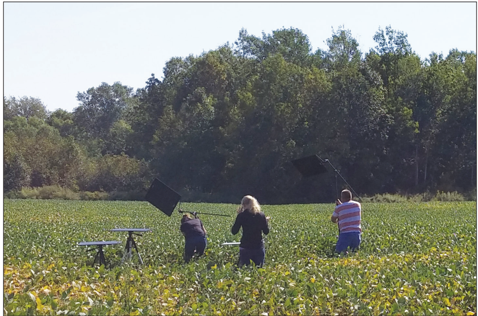
Figure 5: The deployment of calibration panels in a study area enables UAS imagery collected on different days to be scientifically compared, offering crop producers valuable and trusted comparative information. Undergraduate research assistants Elizabeth Bondi and Victoria Scholl assist Professor Carl Salvaggio in a recent experiment at Maier Farms.
