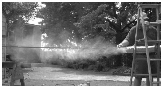
View of Plume during Injection of ~2 micron Particles – Ruler has a 2m scale
