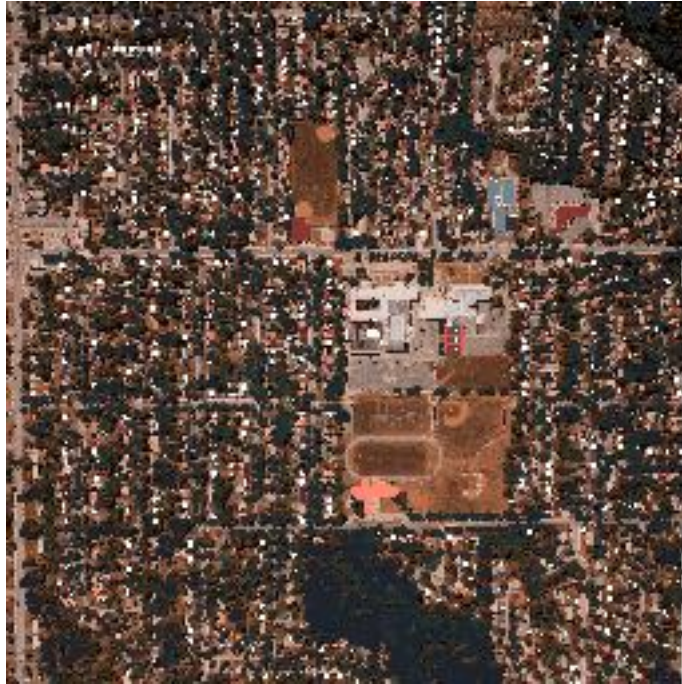
Figure 4.103: This shows the RGB bands when DIRSIG 4 renders the Megascene with a 'realistic' visibility map ranging from 20 to 25 km.
