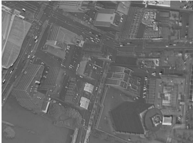
Figure 8: Temporal differenced image produced by subtracting image i_{t1} from the warp created when image i_{t0} was registered to i_{t1} . The image is scaled such that a difference of zero results in a mid-level gray intensity. (Original image courtesy of ITT Exelis WAAS sensor flight test, August 2010.)
