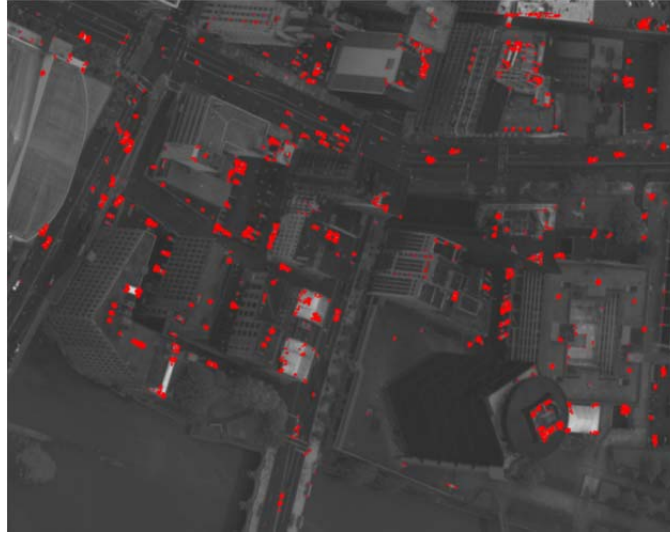
Figure 4: KLT results tuned for feature detection, with a 2-pixel minimum spacing between features and minimum allowable eigenvalue = 150. (Original image courtesy of ITT Exelis WAAS sensor flight test, August 2010.)
