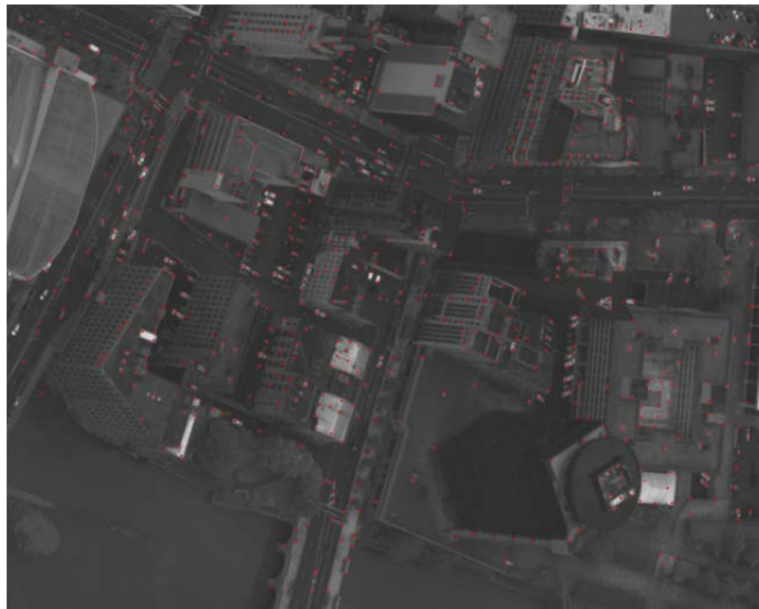
Figure 5: KLT Results tuned for background detection, with a 30-pixel minimum spacing between features and minimum allowable eigenvalue = 300. (Original image courtesy of ITT Exelis WAAS sensor flight test, August 2010.)
