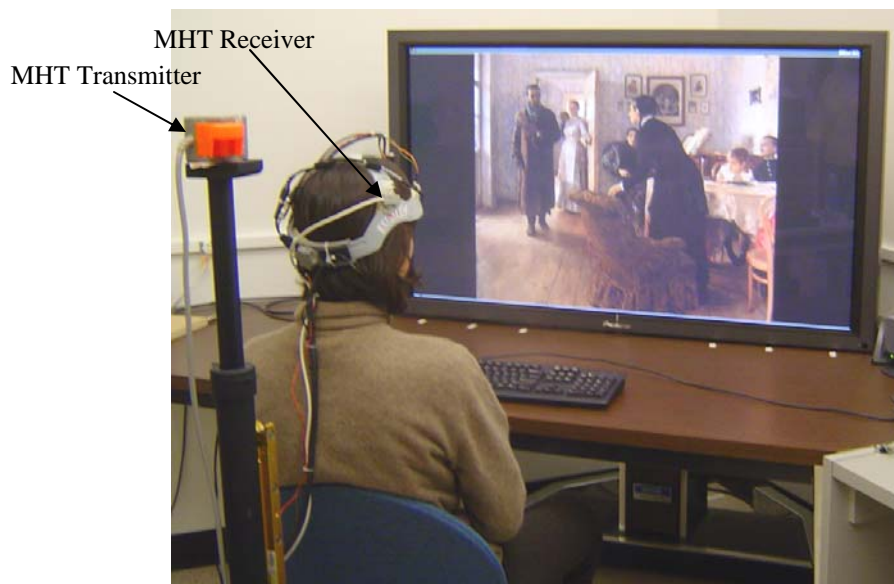
Figure 25: Experimental setup showing the Pioneer 50" Plasma display, the eyetracking headgear, magnetic head tracker transmitter and receiver.
