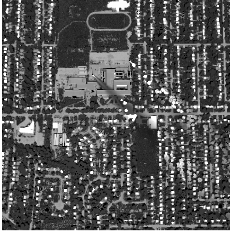
Figure 3.2: Single-band image of Case 2 synthetic DIRSIG data at 10.73\mu m . Both plumes can be seen moving from the middle of the scene to the upper-right corner. The NH_3 plume is the left-most plume while the Freon-114 plume is on the right.
