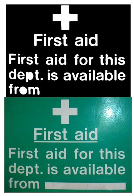
Figure 4.10: Example mostly correct image. Notice some incorrectly filled letters and the incorrect selection of the plus sign. Precision: 0.75 Recall: 0.97 f-metric: 0.85
