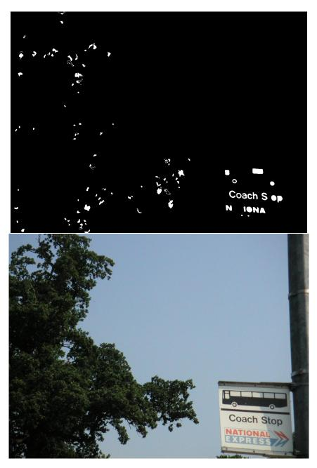
Figure 4.11: Example of a partially correct image. Some text is missing and a significant amount of non-text is incorrectly labeled as text. Precision: 0.36 Recall: $0.29 \ f$ -metric: 0.32
