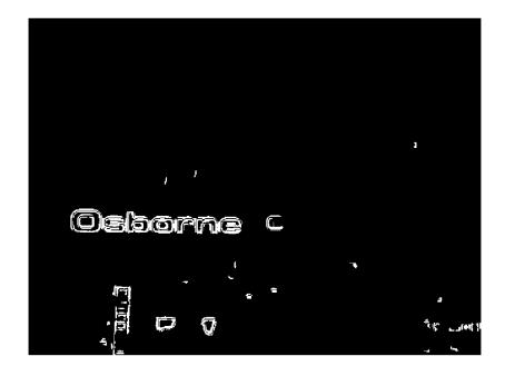
Figure 5.1: Applying a linearity threshold of 0.04 to our sample image results in a significant loss in the text selected.
