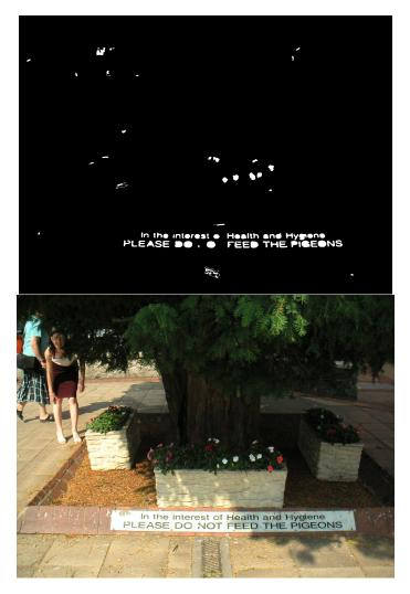
Figure 5.20: In this final example, we see the majority of letters are correctly selected, however there are quite a few false alarms. Adjustment of post processing or the inclusion of OCR may help address this situation.
