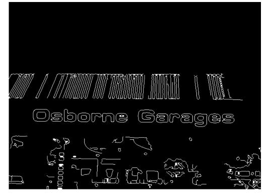
Figure 3.25: Result of running the linearity filter on the Canny edge detection image.
