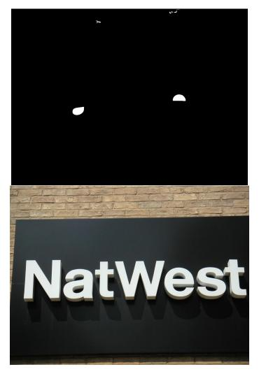
Figure 5.15: Although the classifiers performed well on this image, the Canny edge detector breaks down completely. Adjustment of Canny's parameters may help avoid this issue in the future. Figure 5.16 shows individual components to provide greater detail.
