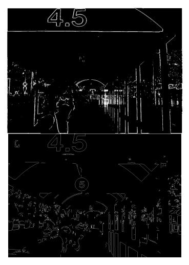
Figure 5.13: Both the sample classifier and the Canny edge detector perform quite well on this image. The issue instead resides in additional post processing steps. This may be corrected by improving post processing and reducing the number of static thresholds used.
