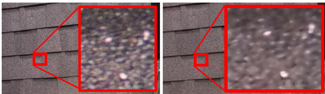
Figure 3.41: Two consecutive pictures were taken from the Phantom 3-4K to show the effects of compression: Left - Uncompressed image. Right - Compressed JPG.
