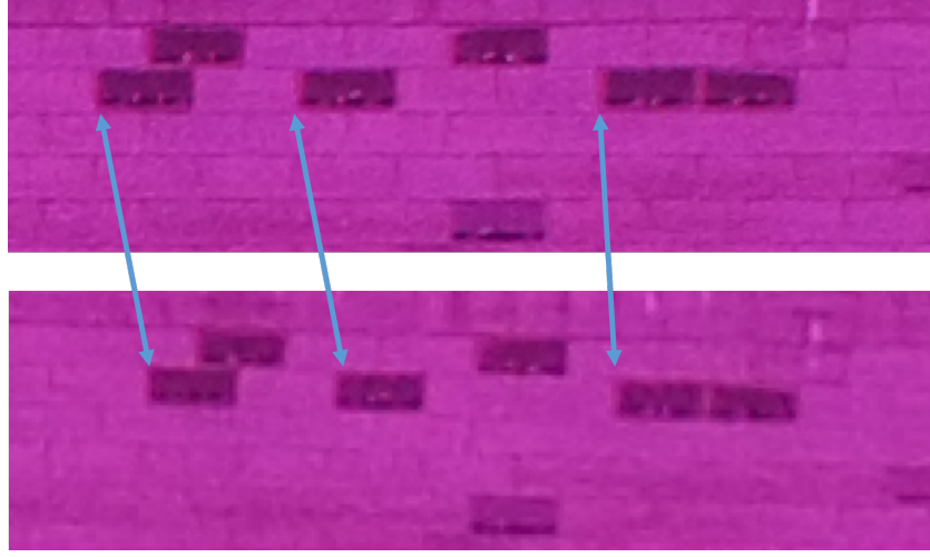
Figure 3.33: Top - Image from 20 m orthogonal flight showing a better resolution, but blur degrades the quality of the image, as denoted by the arrows. Right - Image from the 30 m orthogonal flight has a worse resolution, but blur is not as significant.
