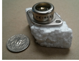
Figure A.1: EK-3431 IR Source with sapphire window
