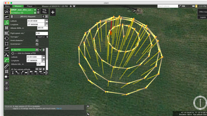
Figure 2.13: Screen capture of UgCS showing a hemispherical flight profile.
