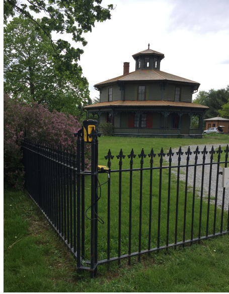
Figure 3.24: Image of reference point E being measured using a Trimble Pro 6h. [Photo provided by Brittany Ambeau.]
