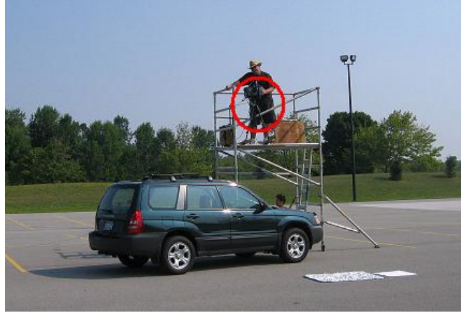
Figure 6.1: Vehicle measurement set-up (red circle indicates the location of the instruments)
