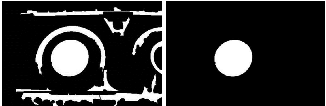
(a) After the flood fill operator was applied
