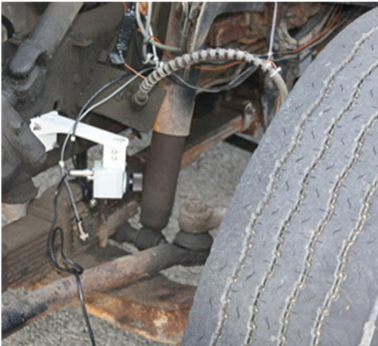
Figure 4.9: Location of the thermal imagers installed in the front, driver side wheel-well of the truck, directed at the front brakes
