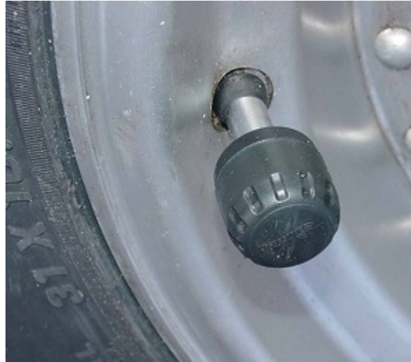
Figure 4.13: One of the six wireless tire pressure monitors that were used to monitor tire pressure
