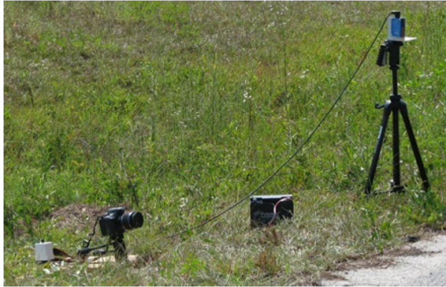
Figure 4.29: The camera and laser trigger used to capture images of the test vehicle's tires while moving
