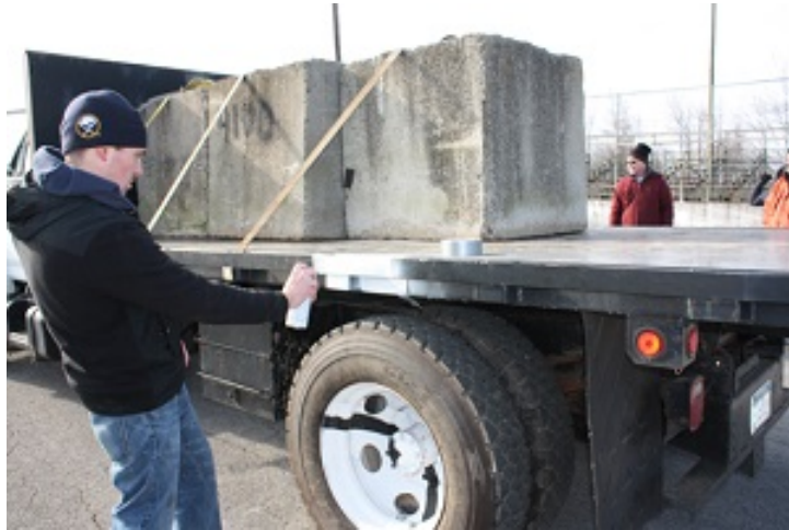
Figure 4.19: A fiducial marker being added to the frame of the test vehicle
