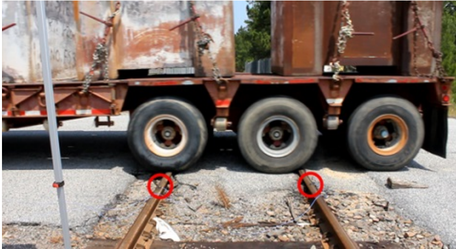
Figure 4.31: The vibration response test in progress for the test vehicle loaded with 40 tons, the circles mark the locations of the accelerometers
