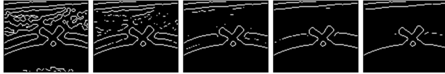
Figure 3.9: An array of binary, edge images generated by varying the contrast stretch (mild contrast stretch on the left to severe contrast stretch on the right)
