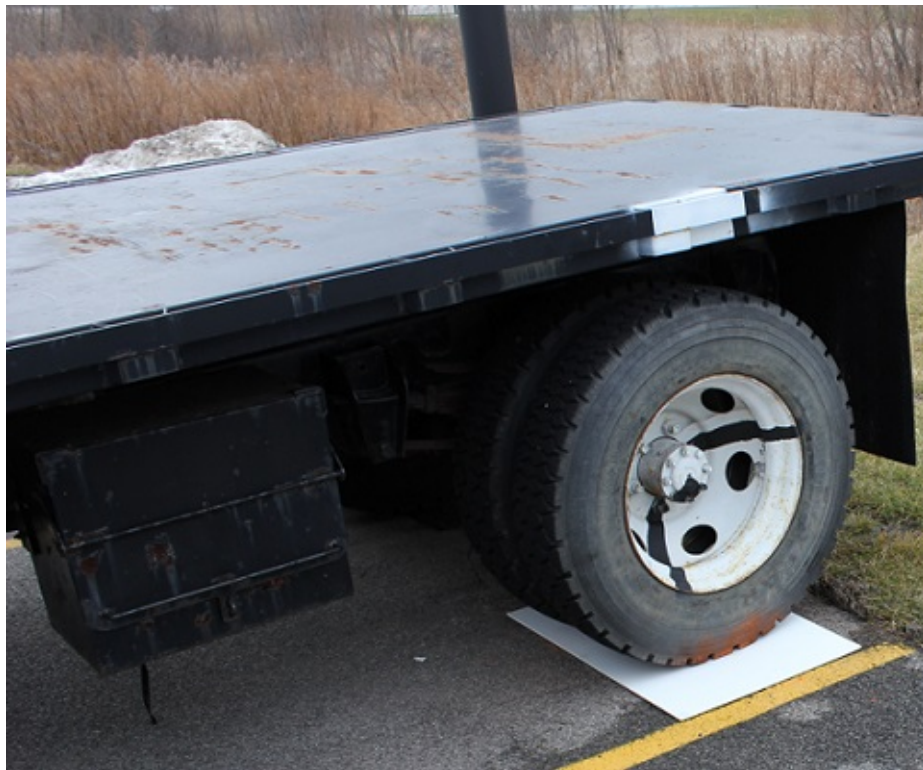
Figure 4.35: The rear tires of the test vehicle positioned on foam-board prior to measuring contact area
