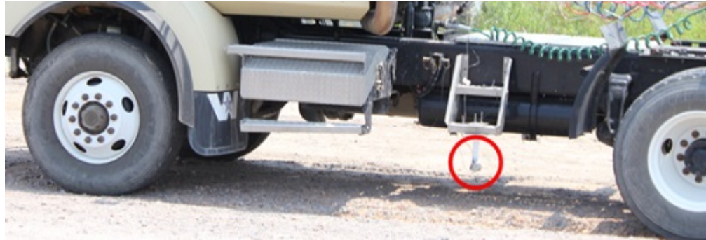
Figure 4.23: Location of the thermal imager installed on the front driver's side of the tractor directed at the front passenger's side brakes and tire
