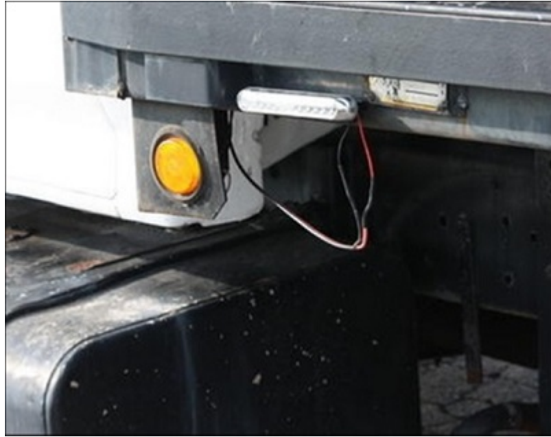
Figure 4.14: One of two LEDs installed on the bed of the truck which were used to synchronize the data collected by the off-board system with the data collected by the on-board system
