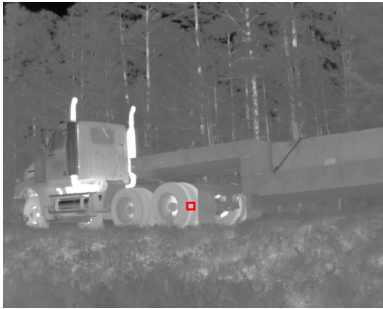
Figure 5.22: Location of the area-of-interest used in the WASP imagery to track the location and calibrated radiance of the hottest region of the test vehicle's tire tread.
