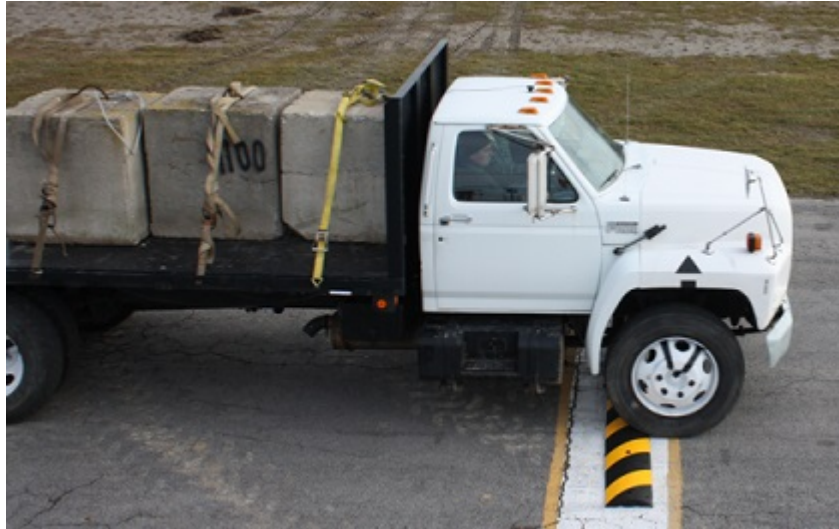
Figure 4.20: The suspension response test in progress for the test vehicle loaded with 3 concrete blocks
