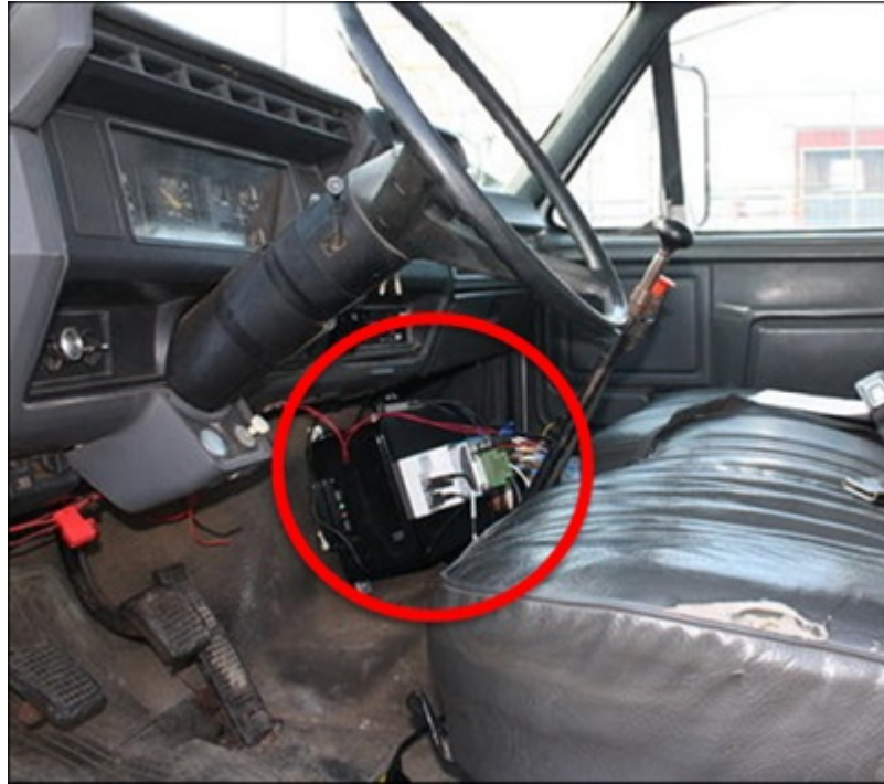
Figure 4.15: The computer and data acquisition system installed in the cab of the truck
