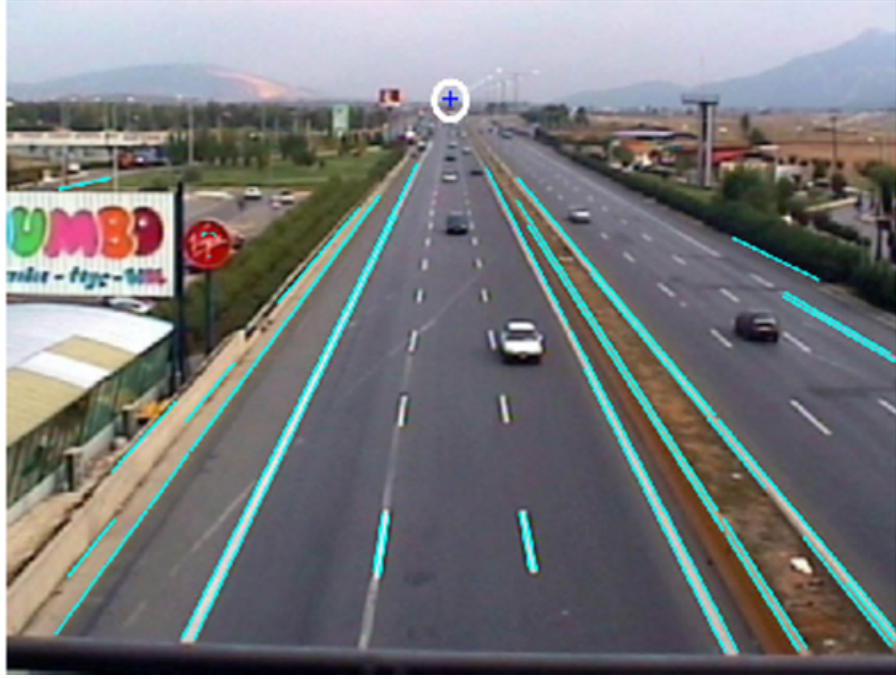
Figure 3.1: Imagery taken using an uncalibrated camera system, highlighted in the image are the lines used to determine the vanishing point and the location of the vanishing point [3]
