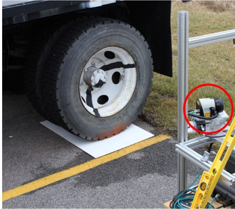
Figure 4.34: The LiDAR system position and orientation used for the first small-scale experiment
