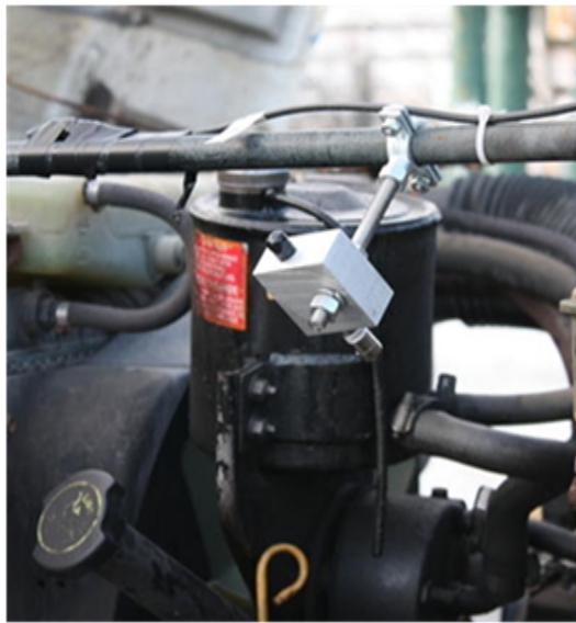
Figure 4.11: Location of the microphone installed in the engine compartment directed at the valve train
