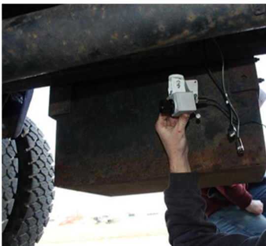
Figure 4.8: Location of the thermal imager installed on the rear of the truck, directed at the rear brakes
