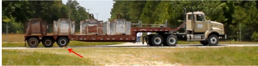
Figure 4.30: The suspension response test in progress for the test vehicle loaded with 40 tons, the arrow marks the location of the speed bump
