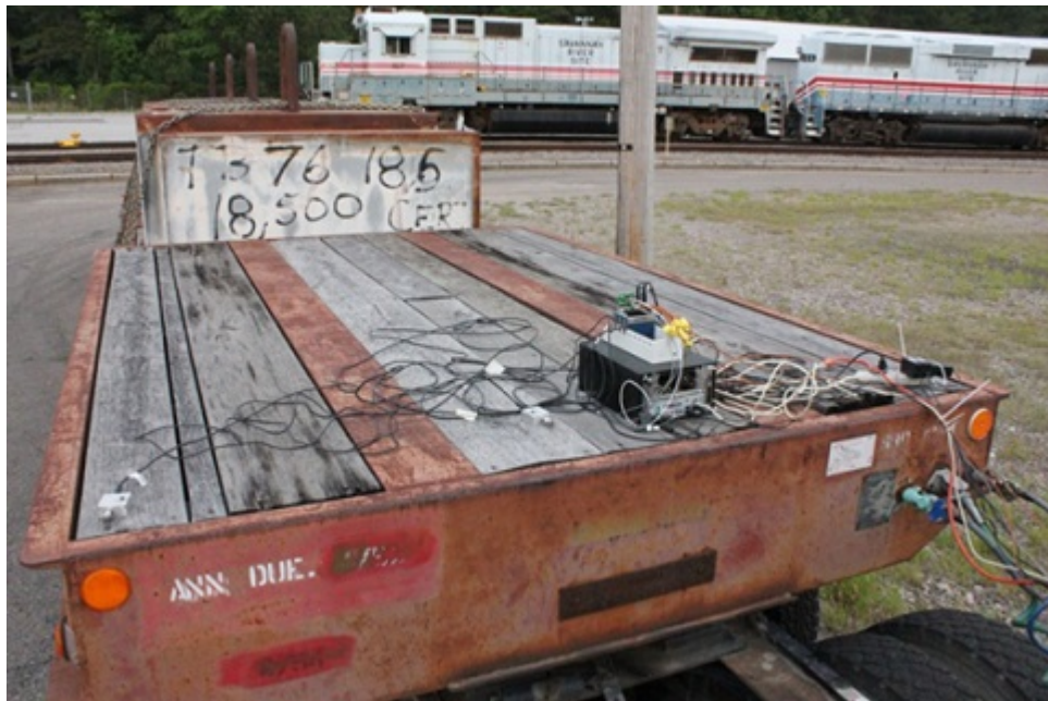
Figure 4.26: The computer and data acquisition system installed on the test vehicle's trailer
