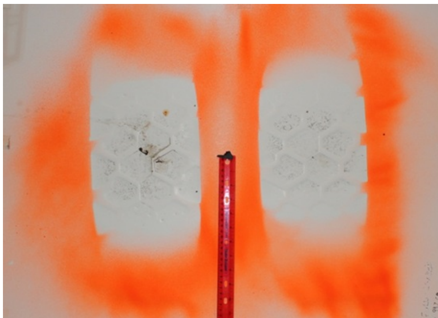
Figure 5.29: An example of a tire footprint outline, measured by spray painting around the perimeter of the tire
