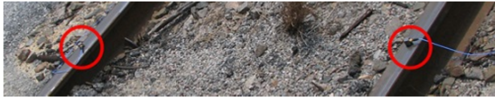
Figure 4.28: Location of the triaxial accelerometers that were mounted on the railroad tracks
