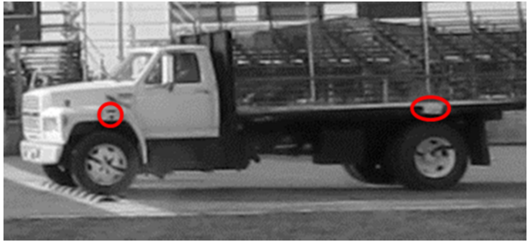
Figure 5.55: Off-board video collected of the test vehicle traveling over the speed bump; the fiducials added to the frame of the test vehicle are circled in red. Fiducials can also be seen on the wheels of the test vehicle.
