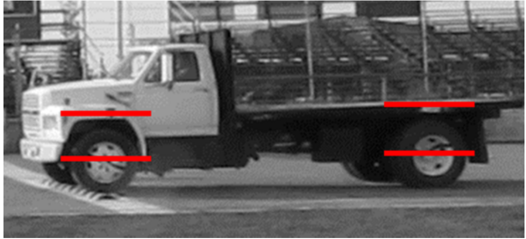
Figure 5.56: Off-board video collected of the test vehicle traveling over the speed bump, the suspension response (the distance between the frame and the fiducial) is marked in red.
