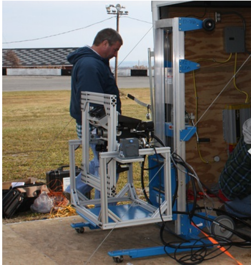
Figure 4.16: The WASP system setup to monitor the test vehicle
