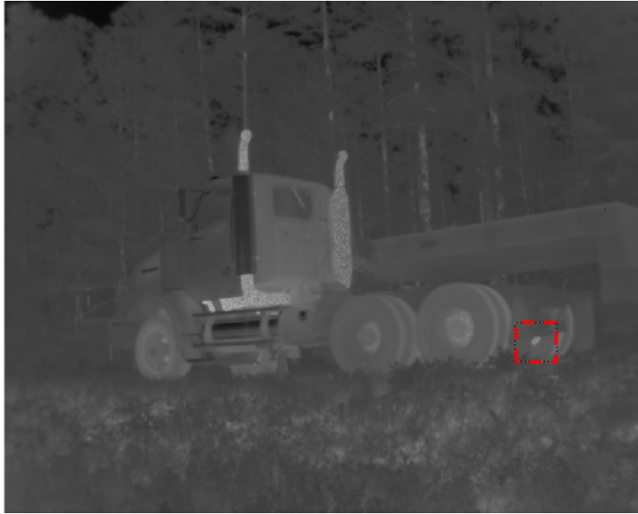
Figure 5.9: Location of the area-of-interest used in the WASP imagery to track the location and radiance of the hottest region of the test vehicle's brake.
