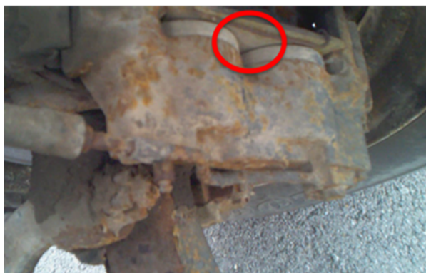
Figure 4.5: The location of the thermocouples installed on the front brakes
