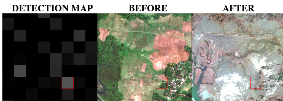
Figure 4.14: Change detection results on an inland region of Indonesia showing tsunami damage to a crop region.
