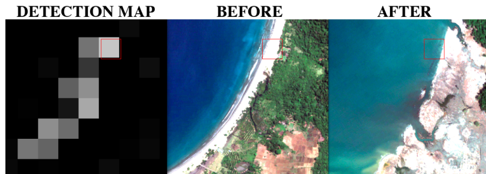
Figure 4.12: Change detection results for an area of significant coastal damage in Indonesia.
