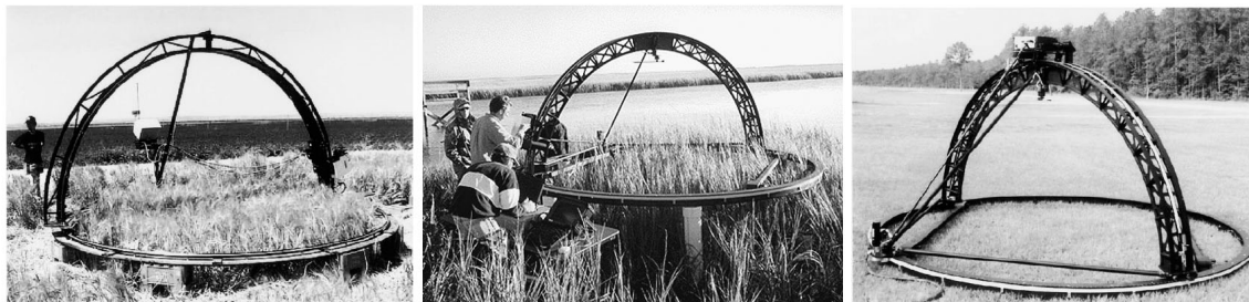
Figure 2.8: An example of field goniometers for BRDF measurements. FIGOS is shown on the left and the SFG system in the middle and right. From Sandmeier [30] ( left and right ) and Schill [35] ( middle ) with permission [36, 37].
