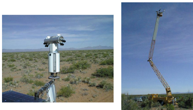
Figure 2.9: The Parabola III system showing the sensor, and the sensor mounted on a boom for field measurements. From NASA [41].
